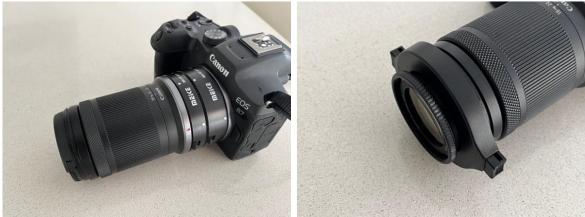
Meike extension tubes (left) and a Raynox DCR-250 converter lens (right) can both be used to turn a regular lens into a macro lens.
